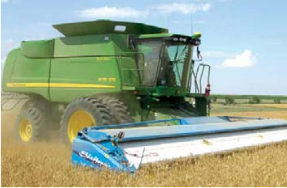
The Shelbourne Header has been developed to reduce the amount of straw being taken into the combine and significantly increase its capacity.
