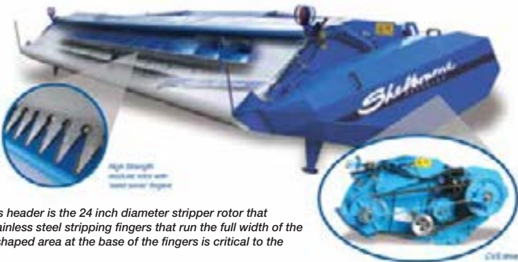
The Shelbourne Header has been developed to reduce the amount of straw being taken into the combine and significantly increase its capacity.
