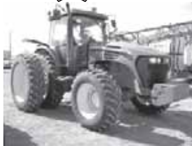
2004 JD 7920, (170 HP), IVT TRANS., MFWD, 3 PT W/ QUIK HITCH, 3 HYDS, PTO, 480/80R46 DUALS
