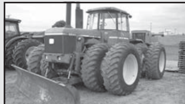
1981 JD 8640 (229 PTO HP) Quad-range trany, 3 hyds, PTO, 3PT hitch, 14' Degelman dozer
