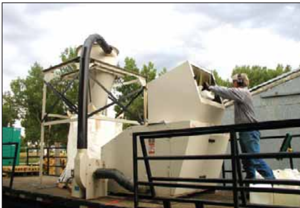
Ron Ahlgren demonstrates how the grinder works to shred plastic pesticide containers. The shredded material then goes to a facility for the manufacturing of drain tiles.
