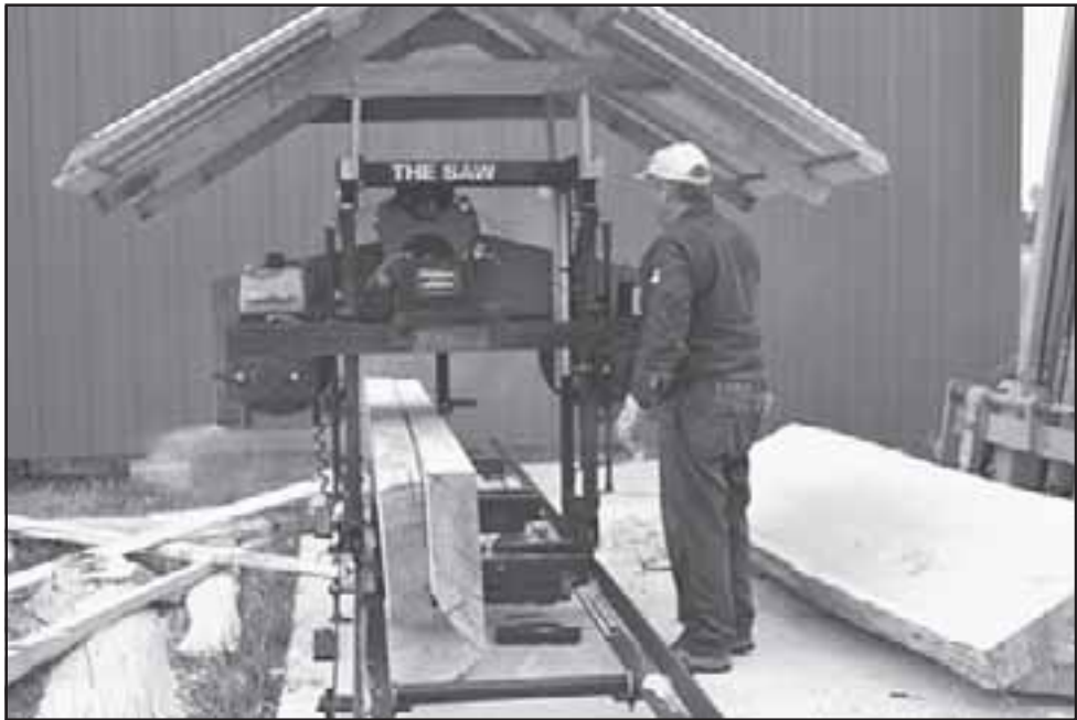
The saw runs on rails, allowing Redman to handle the cutting without assistance.
