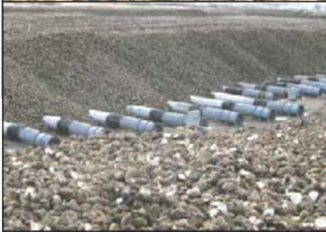
Forced air ventilation helps preserve the beets during campaign.
