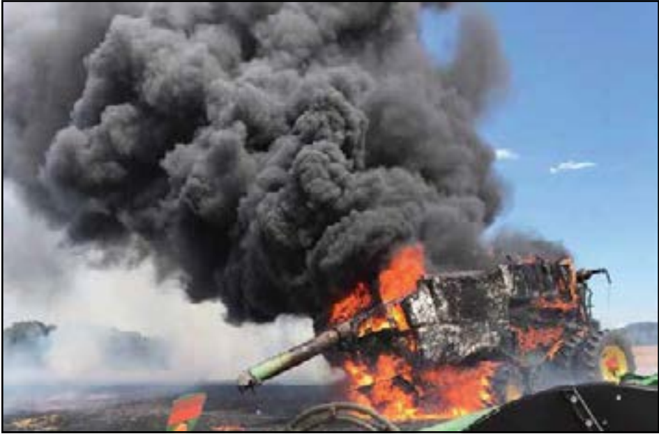
Warm, dry harvest conditions in combination with crop dust and chaff accumulating on hot surfaces can increase the risk of combine fires. (Photo courtesy of Kindred Fire Department)
