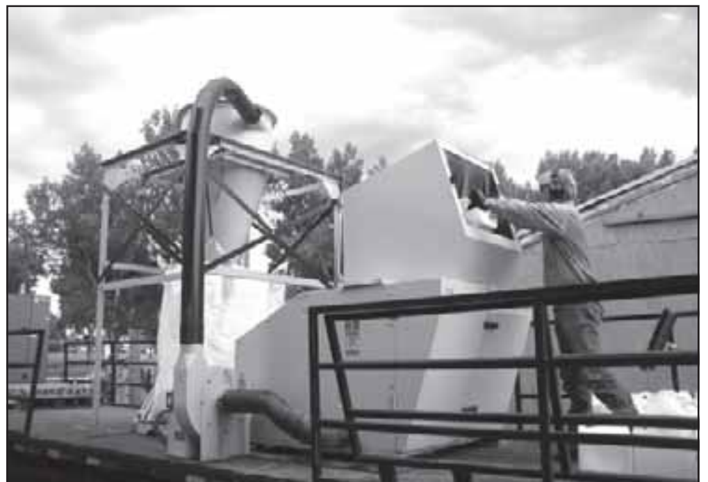
Ron Ahlgren demonstrates how the grinder works to shred plastic pesticide containers. The shredded material then goes to a facility for the manufacturing of drain tiles.
